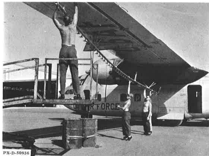
Figure 13. --When insect infestations occur, spraying equipment, including aircraft-mounted types, is used for effective control.
